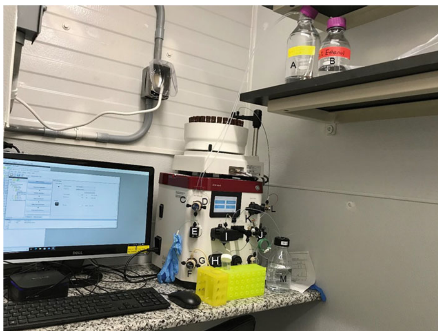
Fig. 2 Instrument modules with annotated parts (a–m): (a) Bottle A; (b) Bottle B; (c) Bottle A attachment to buffer valve; (d) Bottle B attachment to buffer valve; (e) Mixer; (f) Sample valve; (g) Sample valve attachment port; (h) Pump; (i) UV monitor; (j) Injection valve; (k) Column attachment; see Note 16 ; (l) Outlet valve; (m) Waste bottle
